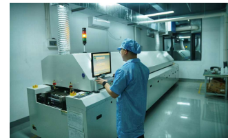
Reflow Welding Test In 10 Temperature Zone
